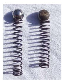
If this valve is worn, it can be the cause of abnormally low oil pressure. It needs to be routinely serviced every 25,000 miles, or when the engine is rebuilt. The valve protects the oil pump by preventing the oil pressure getting too high. This occurs when the engine is cold and the oil is more viscous. The valve is located on the left side of the sump, but is obscured by the chassis rail.
